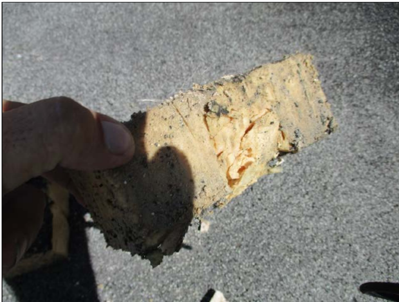
Photo 8: Core location R3, nuke reading 20 – polyiso insulation board.
