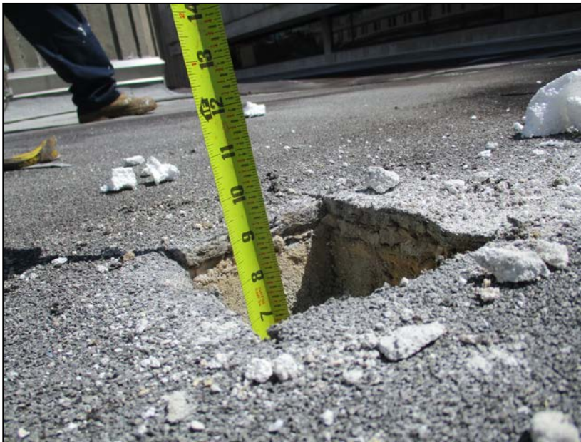
Photo 10: Core location R3, nuke reading 20 – core thickness.
