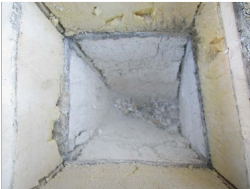
Photo 2: Core location C6, nuke reading 6 – relatively dry.
