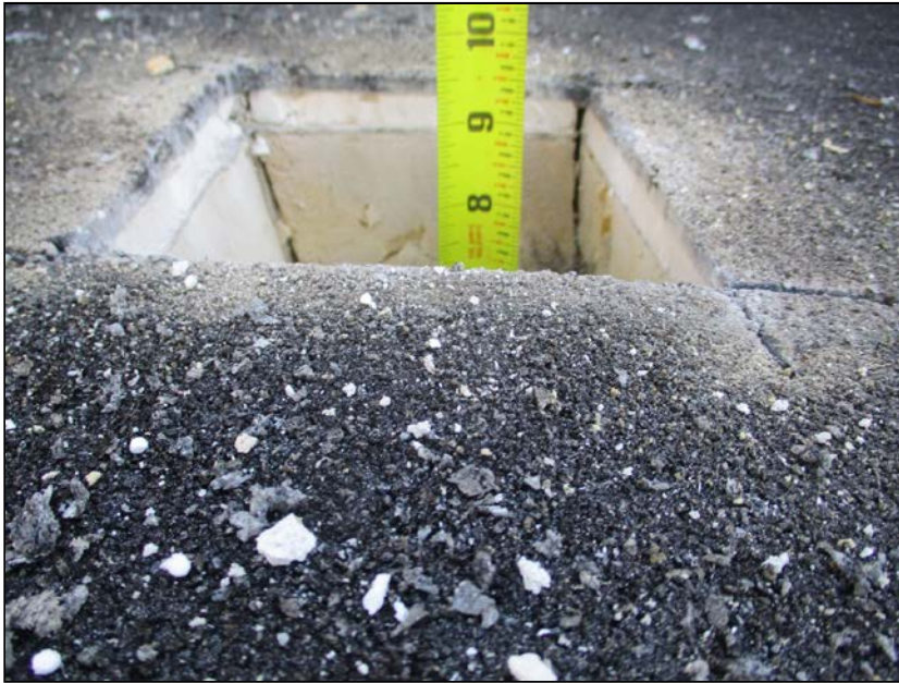
Photo 3: Core location C6, nuke reading 6 – core thickness.
