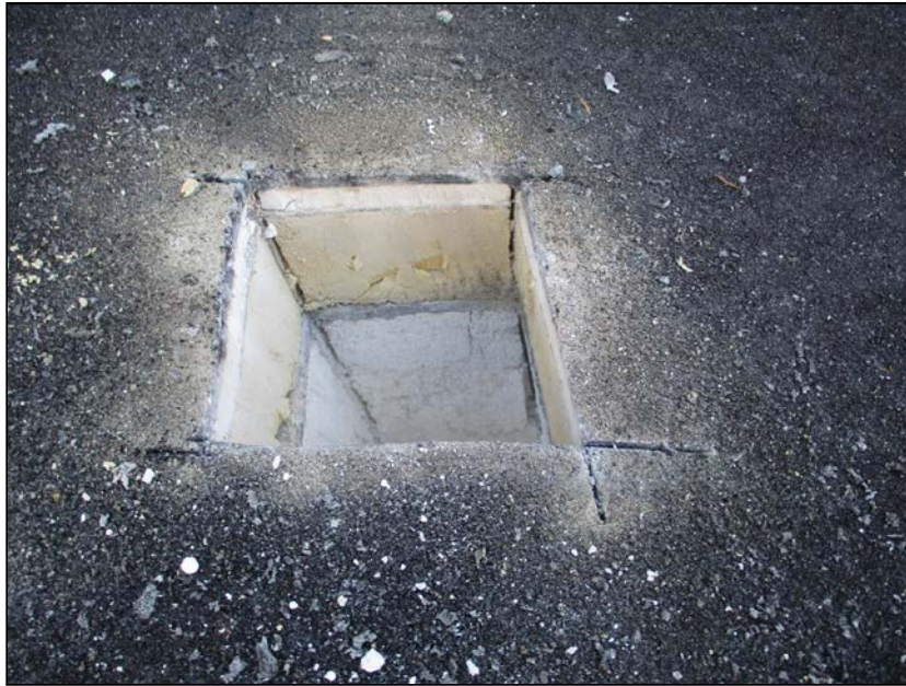
Photo 1: Core location C6, nuke reading 6 – relatively dry.
