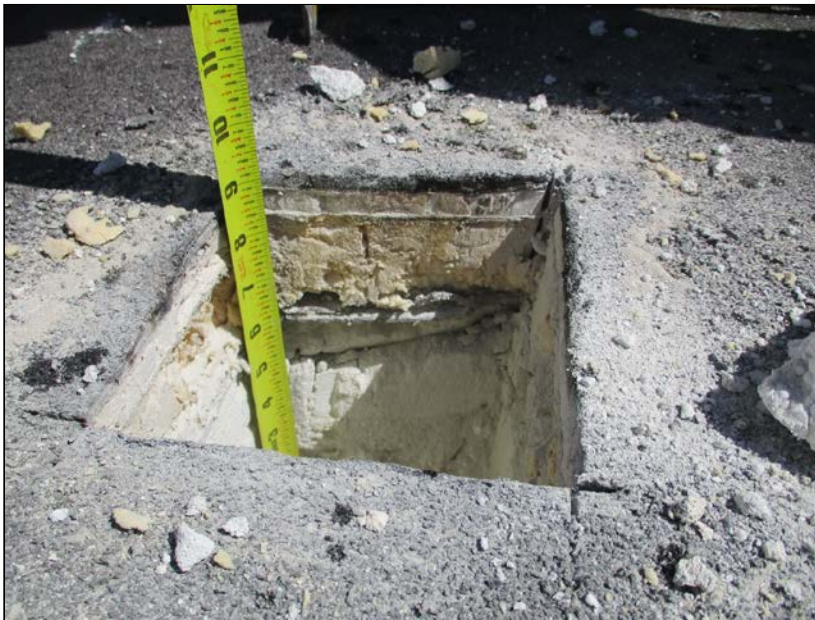
Photo 6: Core location AC5, nuke reading 8 – core thickness.
